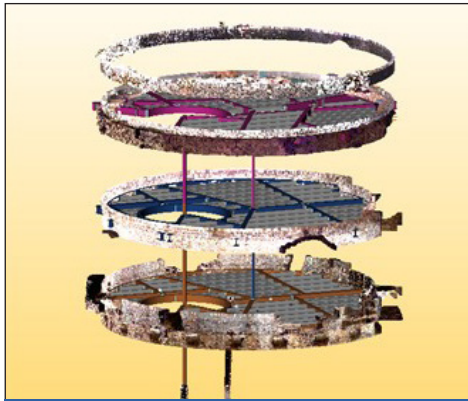
Showing the Tekla .IFC file imported into the point cloud to ensure it was dimensionally accurate
